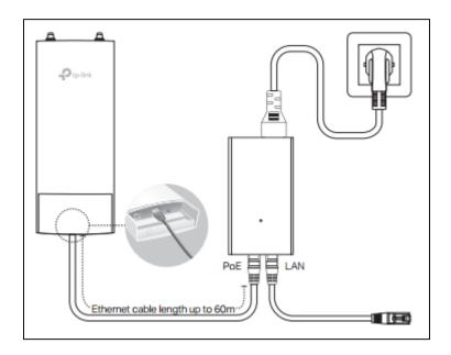
Note: Passive PoE is different from Standard PoE. You cannot supply power to EAP Outdoor products with PoE switches. For detailed information about PoE power supply, please refer to <u>FAQ-906</u>.
